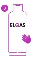
If no line is apparent, run your hand down the cylinder. It will feel cool to the touch at the level of the gas.
