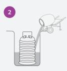
Pour concrete to secure canister in place
