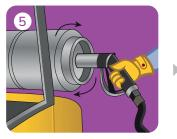
Remove dust cap from cylinder and ensure there are no obstructions or dirt in valve. Connect filler nozzle, turning clockwise and ensuring a tight connection.
