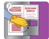
DEADMAN SYSTEM: Latch nozzle in open position then press and hold the dead man's button to start pump and commence fill.
