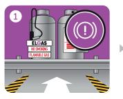
Make sure the forklift is parked safely in the designated area with the handbrake on and the engine turned off.
