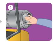
Ensure the forklift cylinder is correctly positioned, with the relief valve at the top. Touch the cylinder to be filled with a bare hand to discharge electricity before putting on protective gloves.
