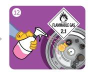
Check cylinder fittings for leaks with soapy water. Replace dust cap on cylinder valve. Do not operate forklift if any leaks present.
