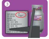
Check LPG cylinder test date. The date stamp must not be older than 10 years and the cylinder must not be damaged by dents or corrosion.
