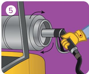
5 Remove dust cap from cylinder and ensure there are no obstructions or dirt in valve. Connect filler nozzle, turning clockwise and ensuring a tight connection.
