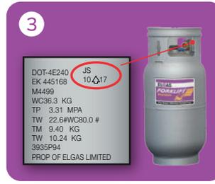
3 Check LPG cylinder test date. The date stamp must not be older than 10 years and the cylinder must not be damaged by dents or corrosion.
